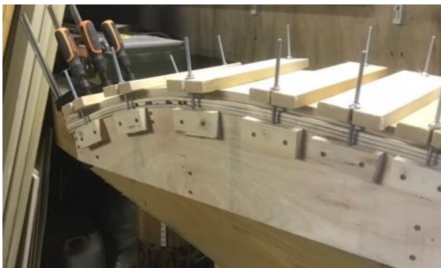
Step 1: bending the case side in a jig
