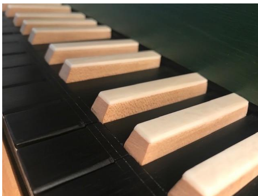
Finished 'reverse' keyboard with ebony naturals and bone (not ivory, honest!) sharps
