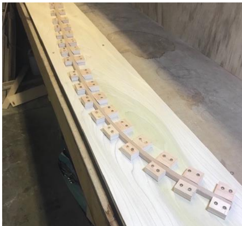
The bridge over which the strings will be stretched is bent to shape
