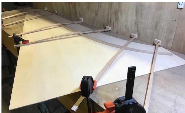
Bridge being glued to the soundboard with bow clamps
