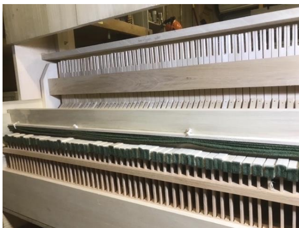
The completed action viewed from the back of the instrument
