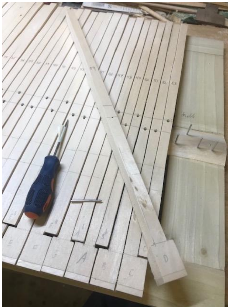
Mounting the keys on their pivot pins
